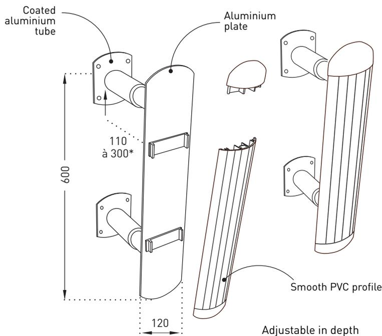
\* A cutting of the tubes is required to obtain an interval from 110 to 256 mm.
