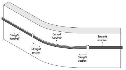
Curved handrails are manufactured using templates manufactured in-situ.
