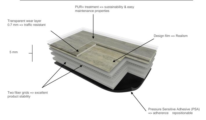
**CREATION 70 X'PRESS** is a synthetic, decorative, flexible, abrasion group T, available in tiles and planks with beveled edges. Composed of a transparent wear layer 0.7mm thick, a design film and three compact underlayers reinforced with two fiber grids, CREATION 70 X'PRESS is 5mm compact product. Compressed and embossed at high temperatures.
