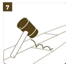
Hammer the planks together, beginning with the small side. Hammer taps must be close to one another to ensure that planks are firmly locked together.
