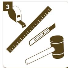
Equip yourself with a ruler, knife, cut-resistant gloves, tape measure, rubber mallet (do not use a metal hammer).
