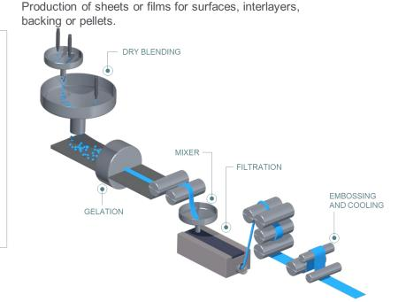
Figure 4: Manufacturing flow diagram
