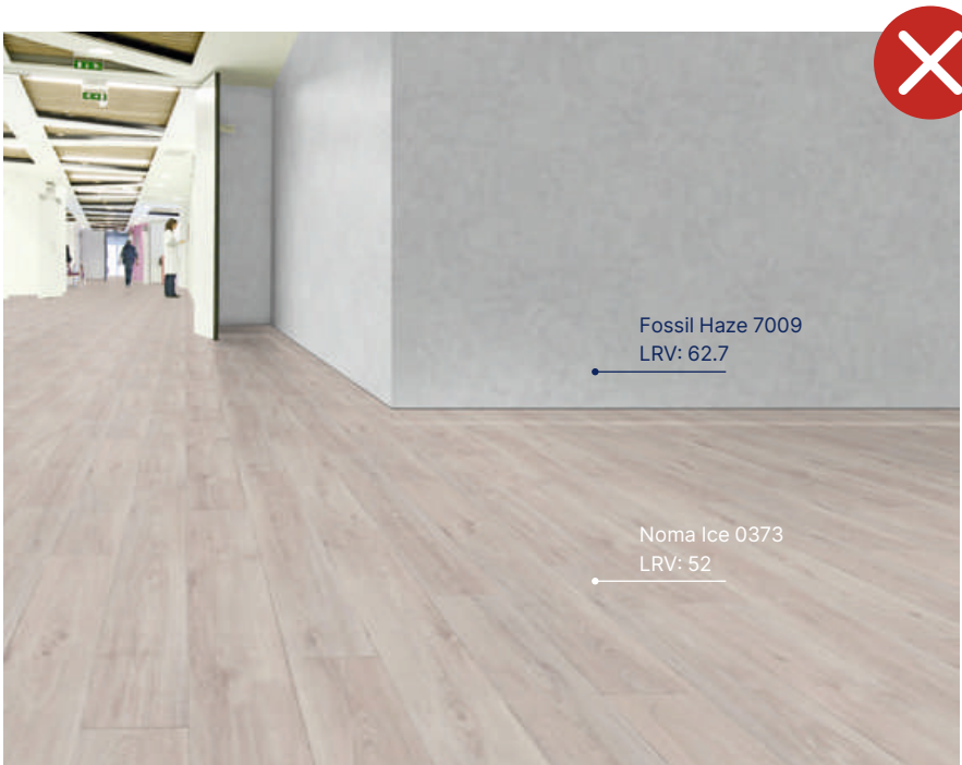
LRV differential of Floor/Wall >30 points
