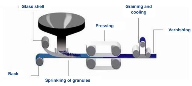
Figure 3: Manufacturing Flow diagram
